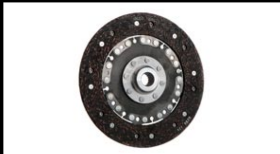
COMING SOON Lotus Sport AP Clutch for Dog Gearbox* 1 Part No. - ALS3Q6016F Applications - S2 (Toyota) Exige when fitted with Dog box AP Racing clutch plate (CP - 5341 - 13) developed for use with the dog box, utilising solid centre plate and improved material.
